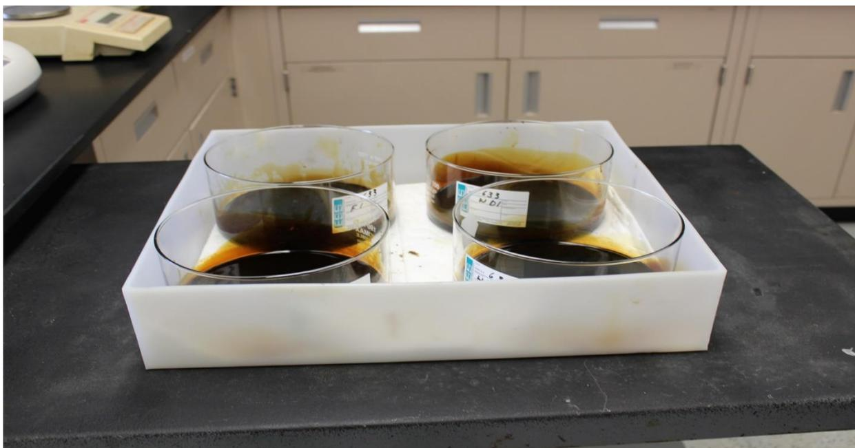
Figure 2. Laboratory weathered HOOPS crude oil samples spread in crystallization dishes ready for rooftop UV exposure.
