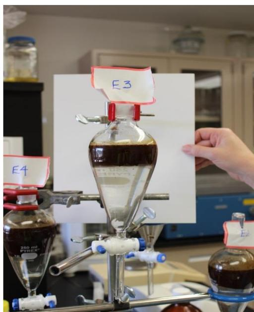
Figure 3. Emulsified oil sample in separatory funnel prior to decanting free water.
