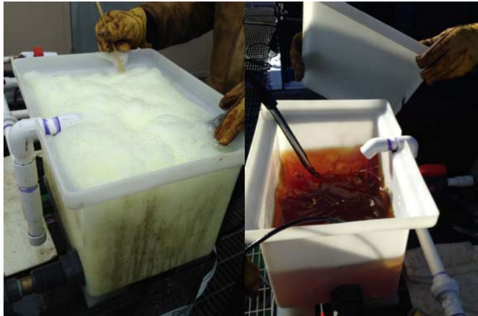
Figure 4 - Comparison of ZI 400 and Finasol while recirculating through the pump and reservoir
