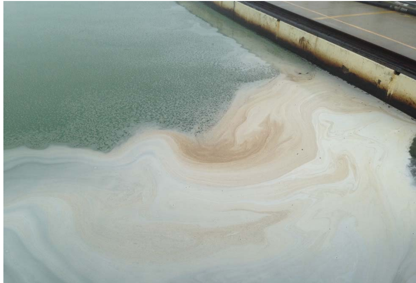
Figure 3 - An example of the foam that appeared after the introduction of Accell to the Ohmsett tank.
