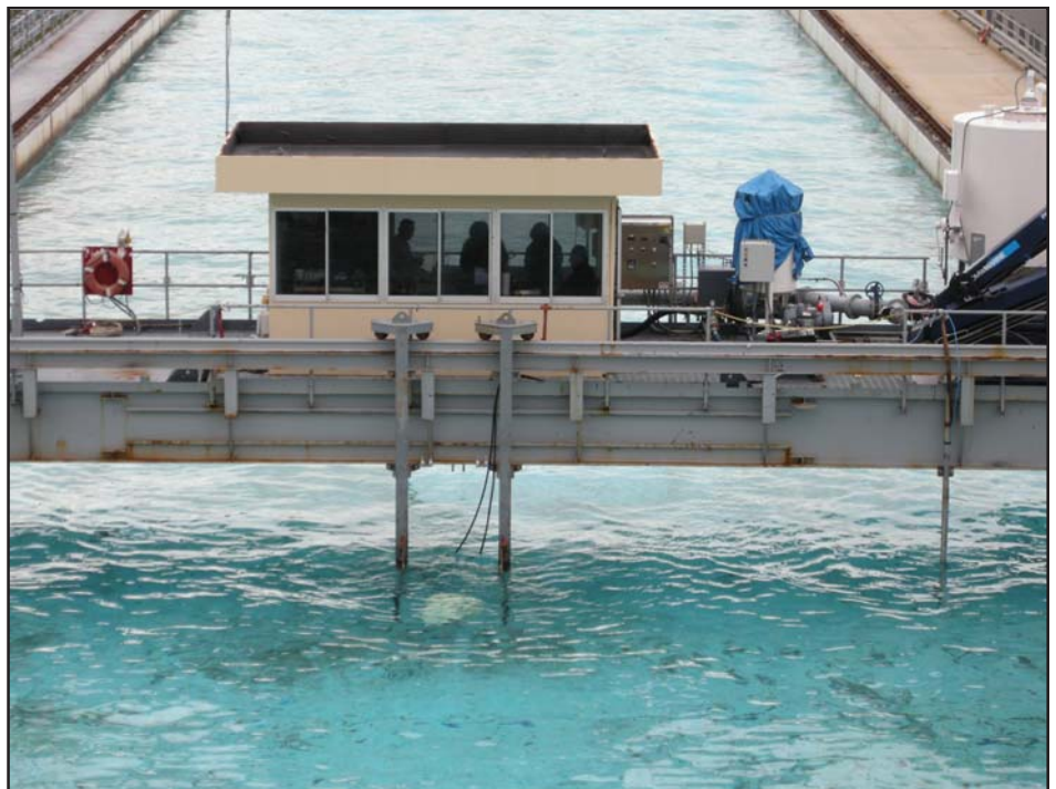
The ECO-Auger™ was mounted to the Ohmsett main bridge and towed through the water. Bridge speed, auger RPM and hydraulic pressure, were measured to calculate horsepower available to drive a generator.
