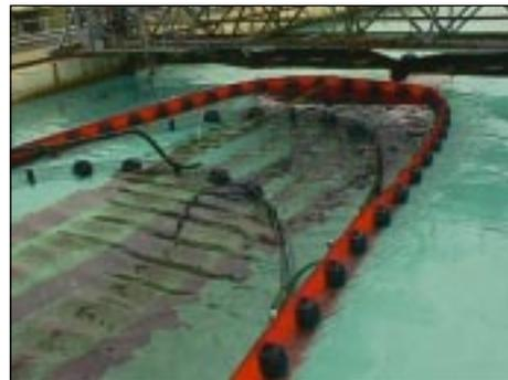
**Exxon's high current oil containment barrier in the Ohmsett tank**
