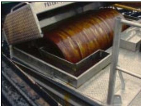
**Goo-Gobbler gobbles up Hydrocal during testing in the Ohmsett tank.**
