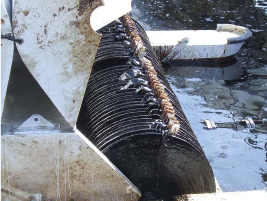
Figure 3: Tests were performed with the oleophilic discs operating at different rotational speeds
