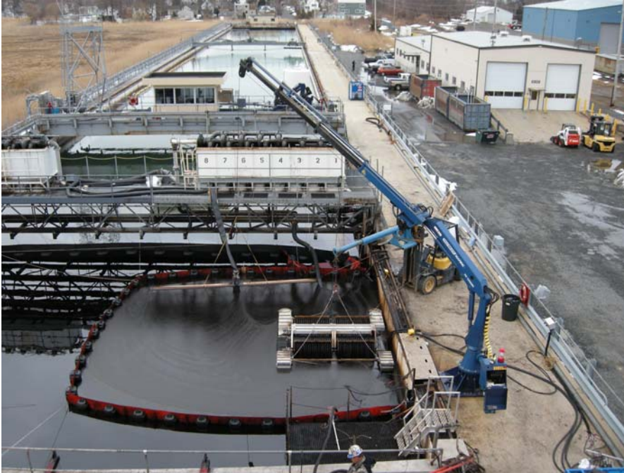
Figure 2: Testing with skimmer adjusted to optimum setting and discharge flow directed to the collection tanks
