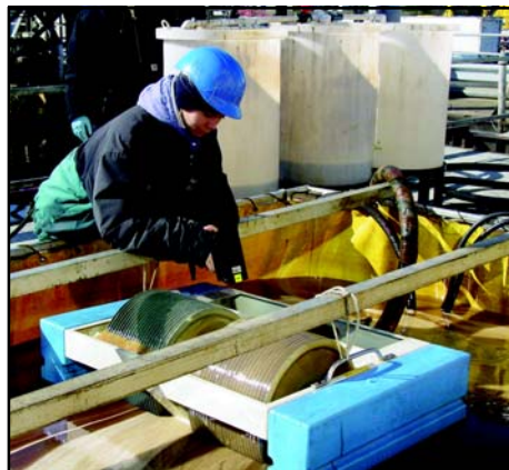
Victoria Broje of Bren School of Environmental Science and Management, University of California Santa Barbara tests oil spill recovery rates during the oleophilic skimmer recovery surface research at Ohmsett.
