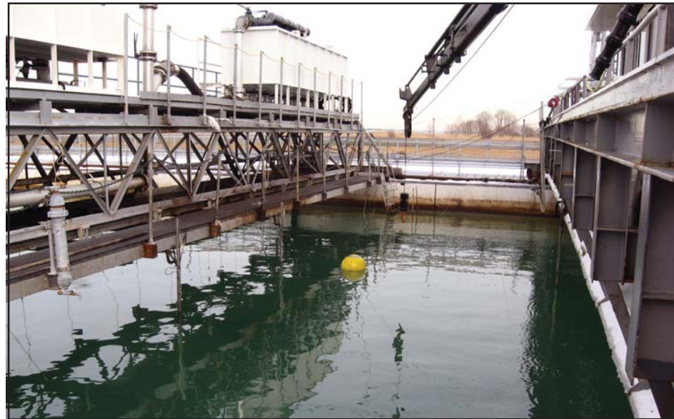
The Resolute prototype wave energy converter was anchored to the bottom of the Ohmsett wave tank while waves were generated in various configurations to determine certain performance characteristics of the device.
