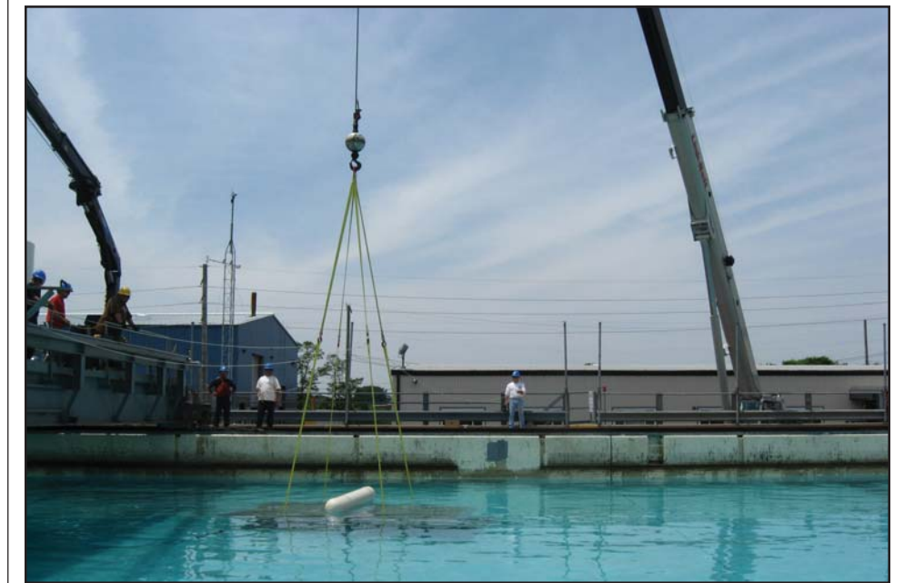
A large crane is used to lower the SurgeWEC into the Ohmsett test tank.
