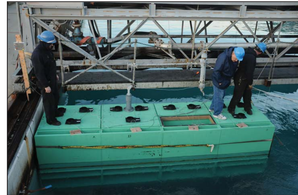
The Rho-Cee wave energy converter can potentially convert wave energy into electricity.
