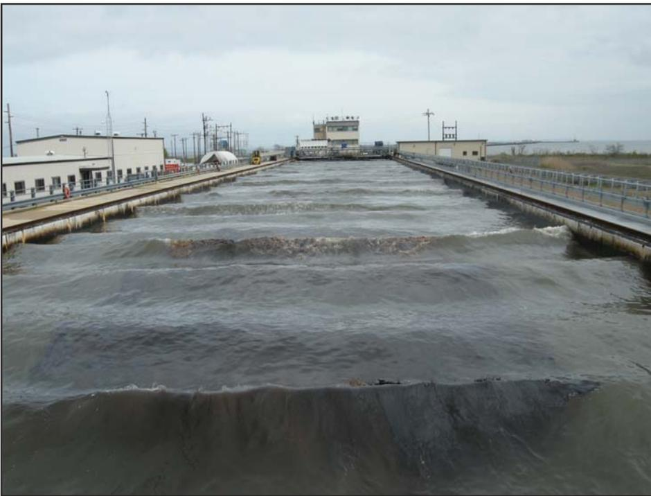
**During the Dispersant Effectiveness Tests in Low-Doses and Repeat Applications, an oil slick was applied to the water and the main bridge was moved over the slick as dispersant was applied in a low dose. Researchers waited a few minutes; then applied another low dose of dispersant.**
