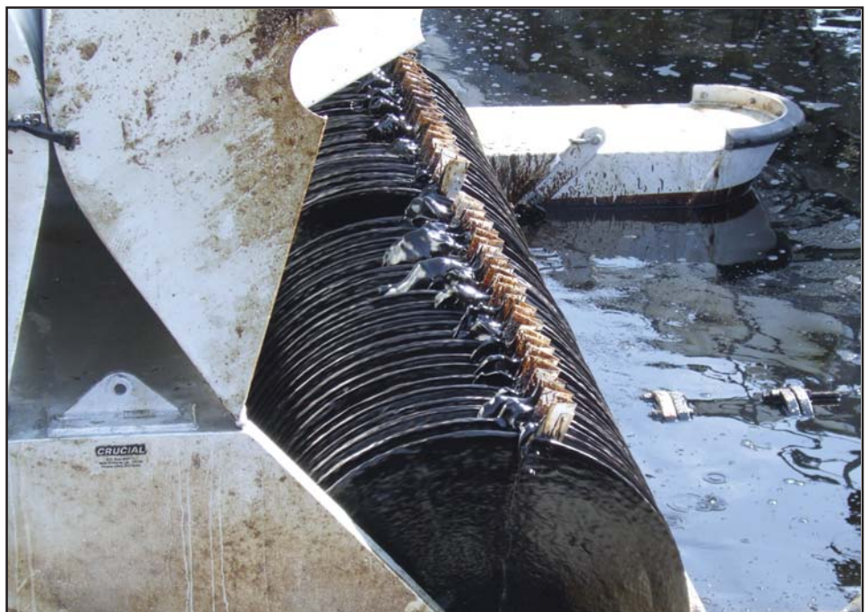
The Crucial prototype skimmer head was tested with fresh and weathered Alaska North Slope crude oil during the test funded by the Prince William Sound Shippers.
