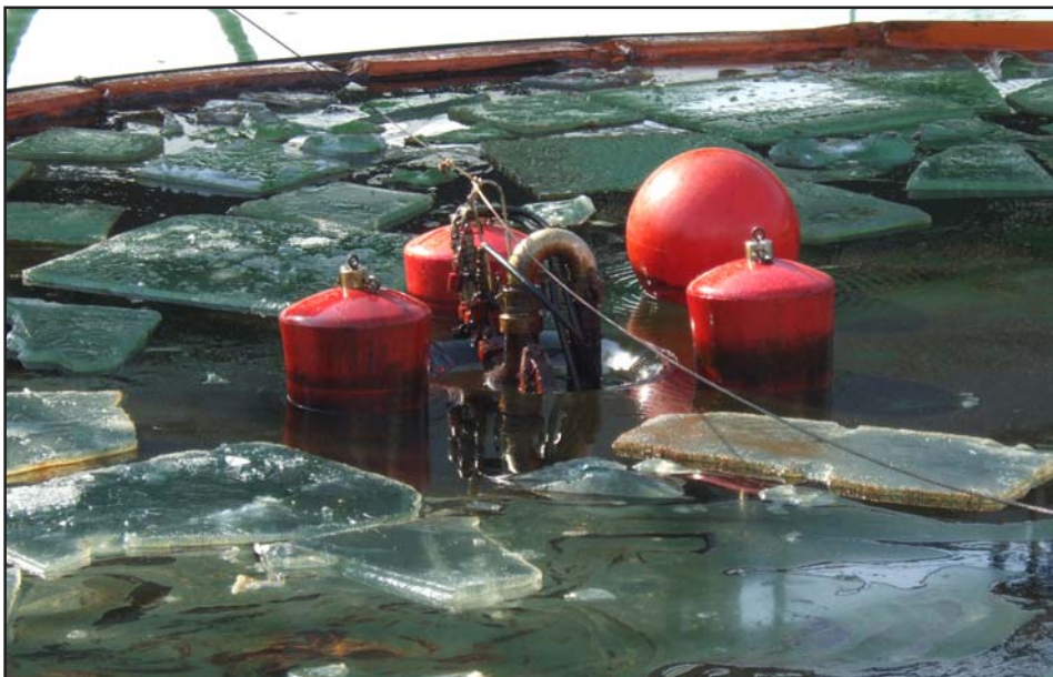
After oil and a herding agent was applied to the controlled test area, a skimmer was used to remove oil from the center of the ice-laden herded oil slick.
