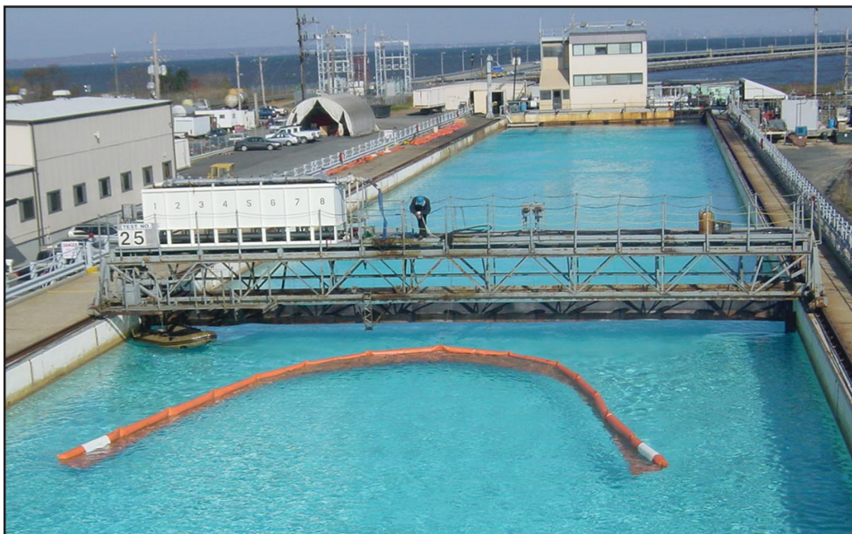
The NOFI Trömso prototype boom system's performance is put to the test
