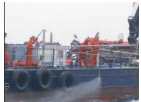
Researchers apply dispersant to a slick in at-sea trials in the United Kingdom.
