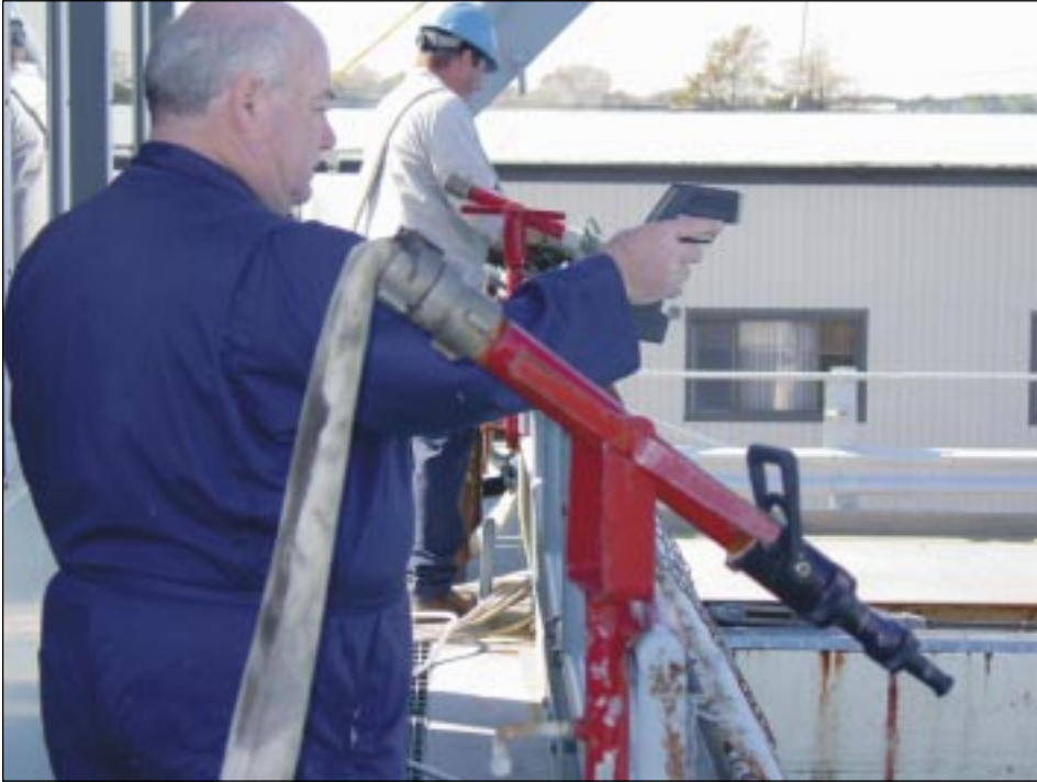
Ken Trudel of SL Ross measures oil temperature with a handheld IR thermometer.
