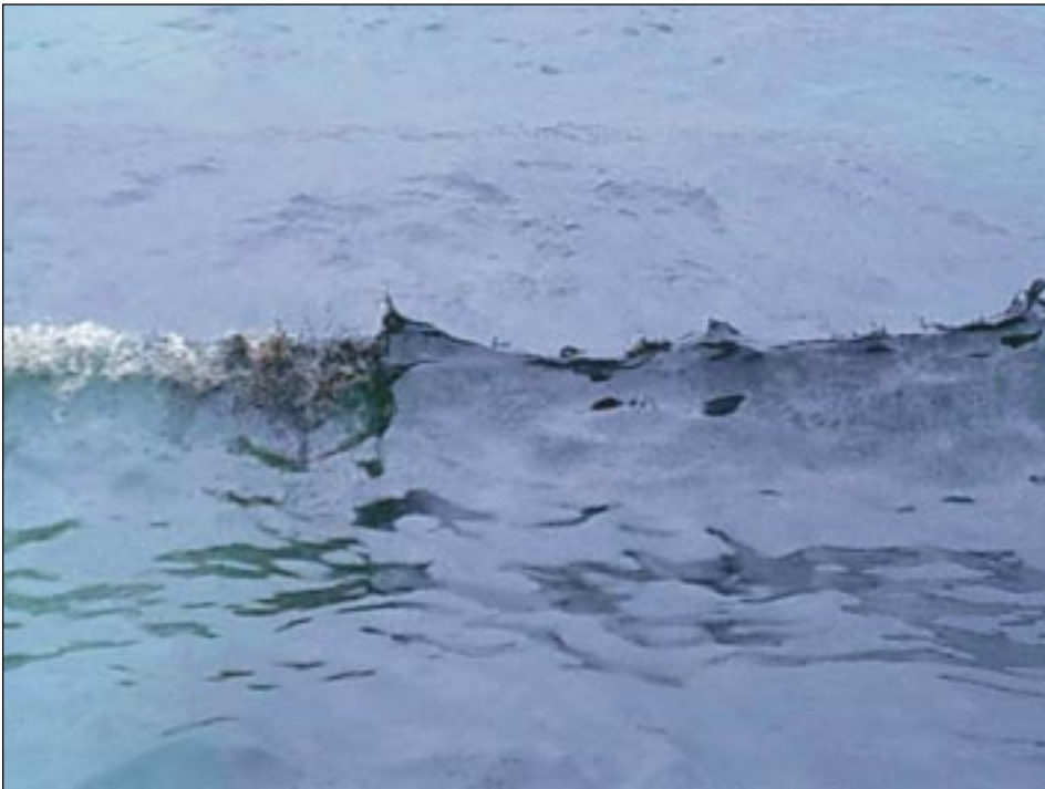
Waves act upon the oil slick and dispersant in the Ohmsett basin.
