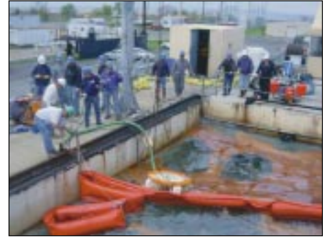
Operating a skimmer in the test basin.
