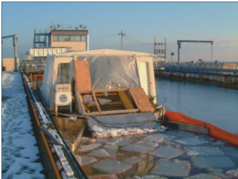
The MORICE skimmer awaits testing at the edge of the Ohmsett test basin.
