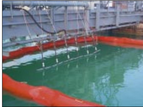
Nozzles are positioned for applying dispersants during testing.
