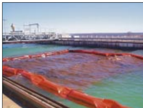
Ohmsett test basin waves mix oil with dispersants.
