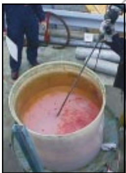
The decanted water and oil are mixed prior to sampling
