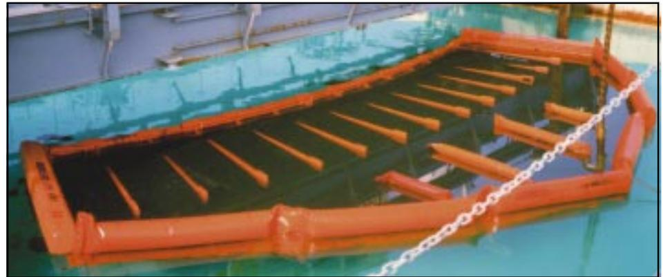
UNH's oil barrier in the Ohmsett tank
