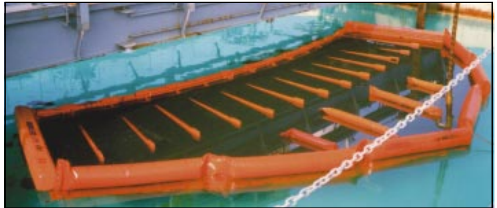
UNH's oil barrier in the Ohmsett tank
