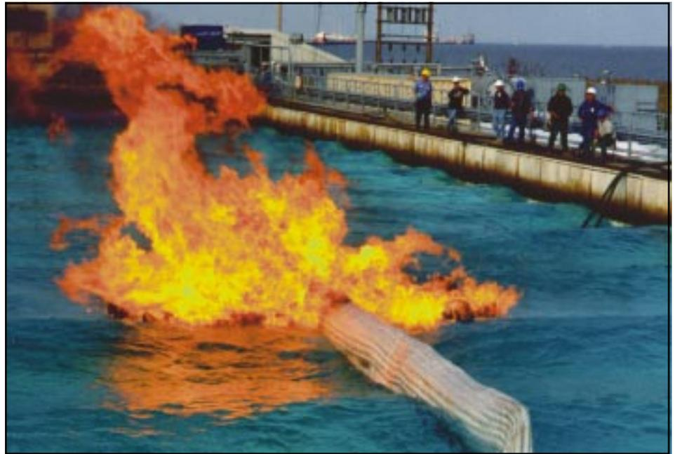
Things really started heating up at Ohmsett in 1998—on the order of about 900 degrees centigrade. In a joint endeavor, SL Ross Environmental Research, GPC, and Ohmsett technicians rigged an underwater propane bubbling system in Ohmsett's tank to test fire-resistant boom blankets in flames.
