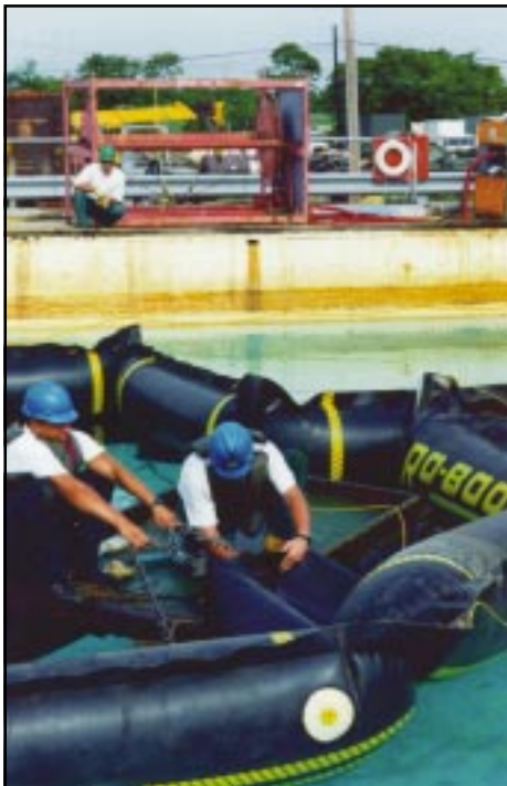
Ohmsett technicians installing sensors
