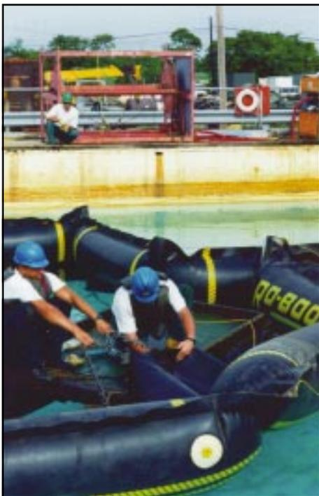
Ohmsett technicians installing sensors
