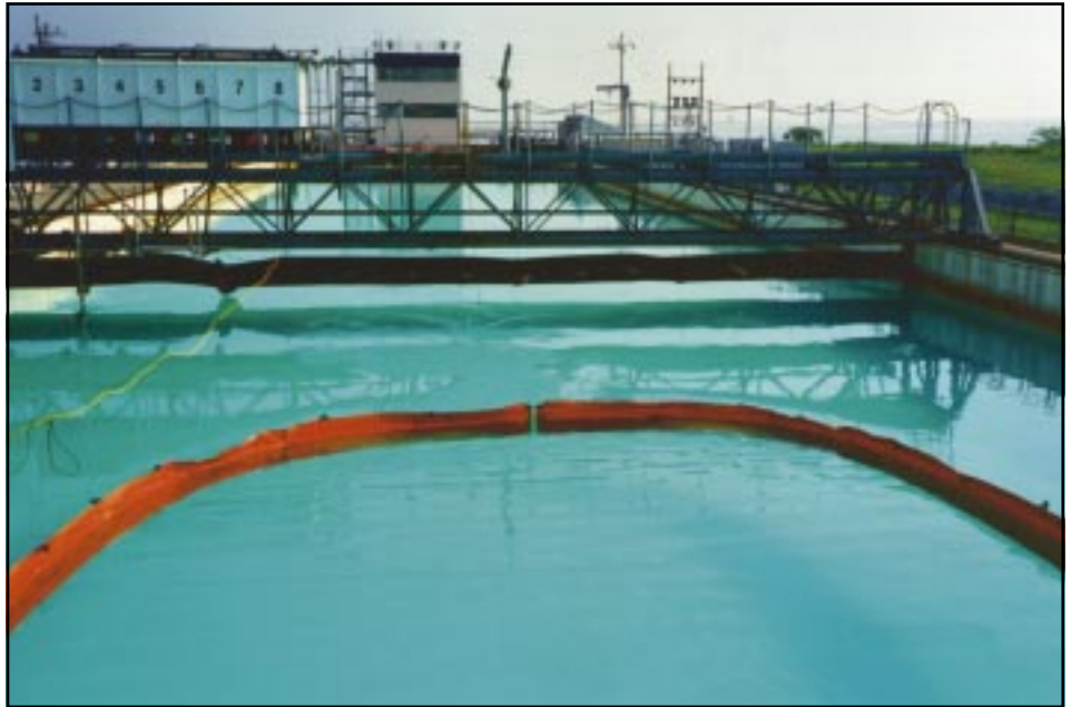
Boom towed in the characteristic "U" shape
