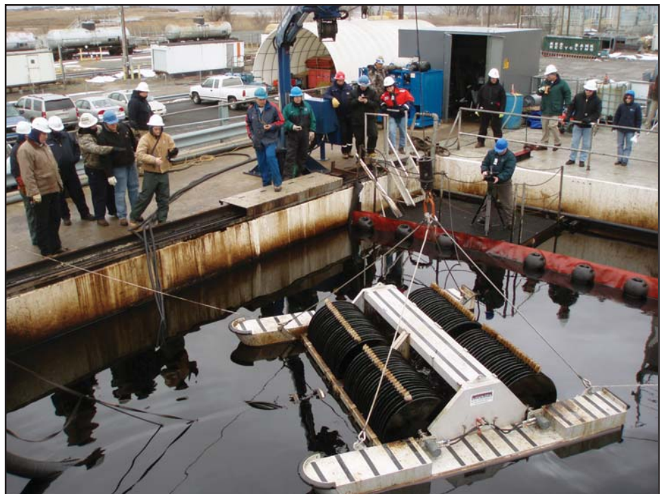
With modifications, the Crucial skimmer prototype was tested to the ASTM Skimmer Protocol to determine the Oil Recovery Rate and Oil Recovery Efficiency. In addition, it endured a 24-hour extended run durability performance test.
