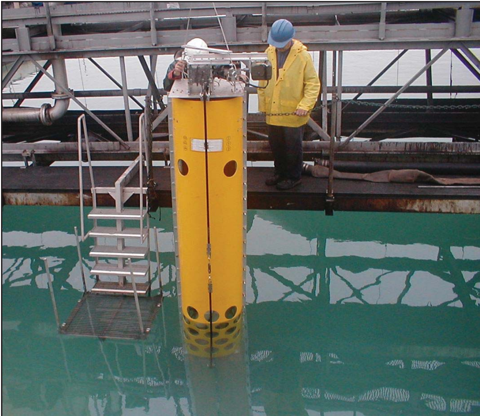
The Electricity Generating Wave Pipe (EGWaP) was placed in the water fitted with probes and sensors that measured the energy output of the device. Waves were introduced to determine its ability to produce energy, as well as its ability to withstand the marine environment.
