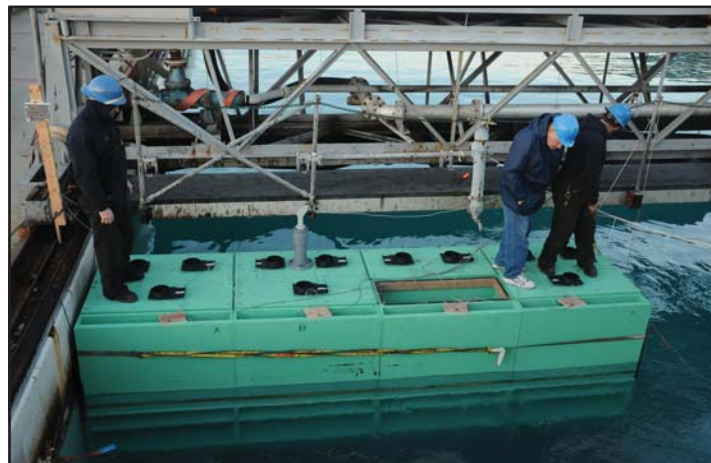
The Rho-Cee wave energy converter can potentially convert wave energy into electricity.
