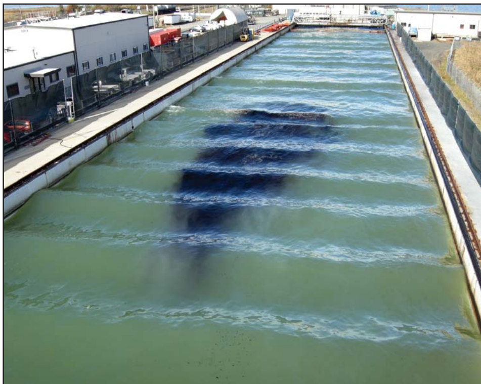
Dispersant tests were conducted in the Ohmsett tank to establish large-scale dispersant effectiveness estimates and to determine if researchers could predict dispersant performance at sea.
