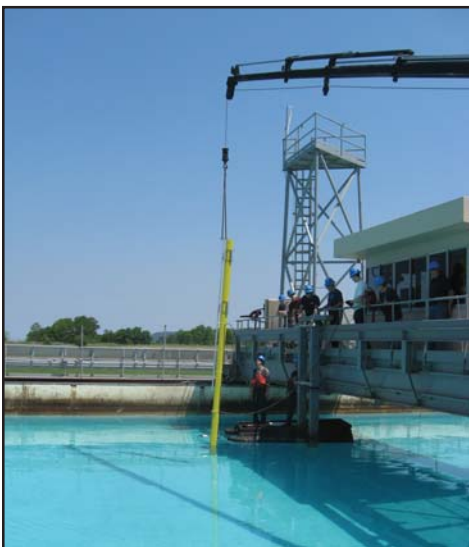
Resolute Marine Energy and Ohmsett built a special-purpose spar to house the instruments needed to measure wave height, wave period, water particle motion, etc., during the evaluation of the SurgeWEC prototype.
