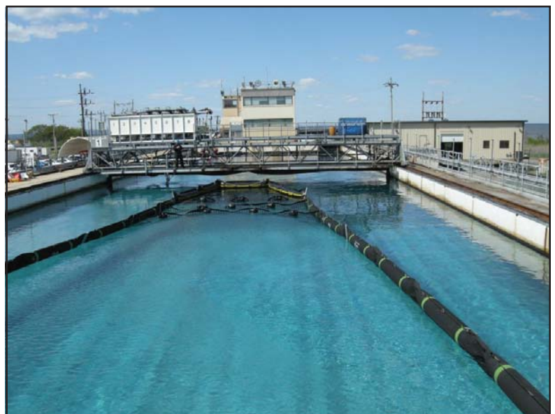
The OilShaver prototype is tested with oil in calm water conditions in the Ohmsett test tank.
