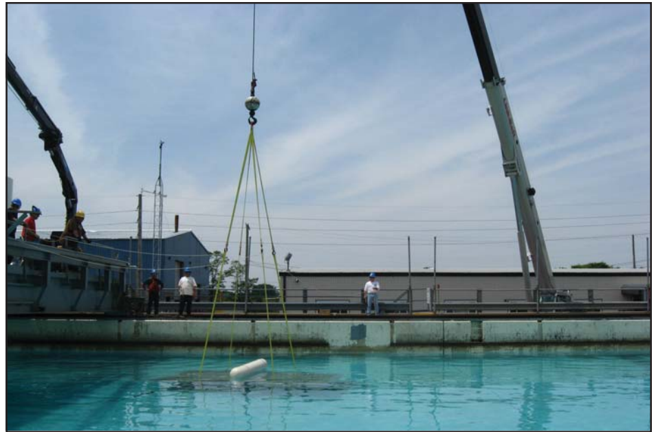
A large crane is used to lower the SurgeWEC into the Ohmsett test tank.
