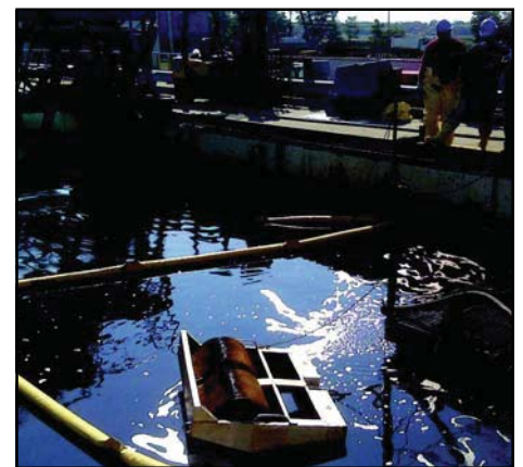
During the Swift Water Spill Response course, students practiced deploying a drum skimmer.
