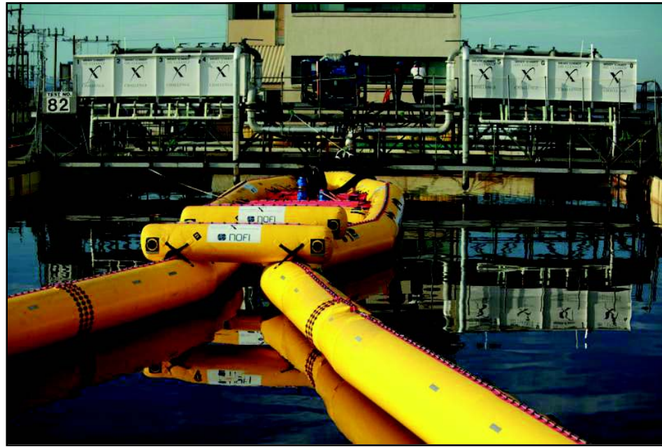
Second Prize winner, Team NOFI with their single vessel unit, the Current Buster 6. The system's recovery rate was 2,712 gpm at 83 percent efficiency.
