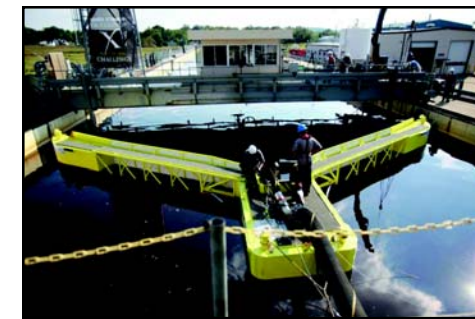
Koseq's floating steel system with a V-shaped arm is towed through the water.
