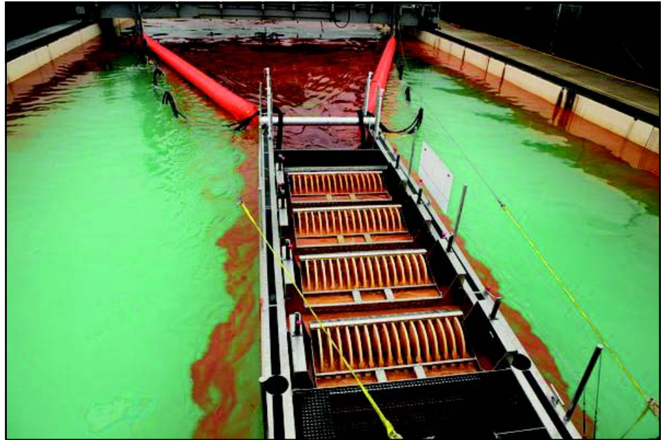
The Wendy Schmidt Oil Cleanup X CHALLENGE First Place prize winner Elastec/American Marine oil-skimming system with four rows of rapidly spinning grooved discs achieved 4,670 gallons of oil per minute at 89.5 percent efficiency.
